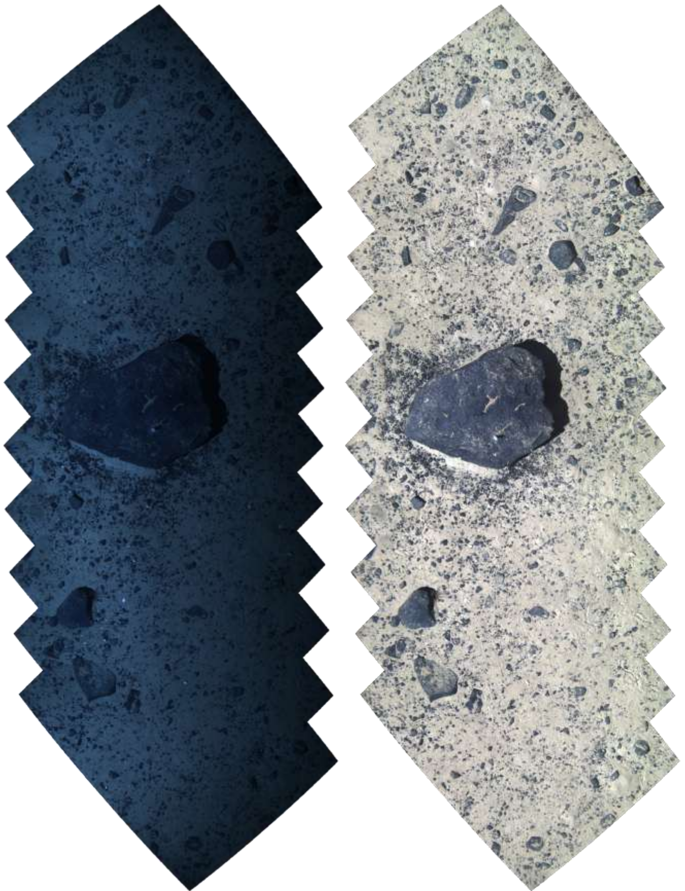
Figure 7. Raw (left) and corrected (right) photomosaics of a sequence of 10 images.
