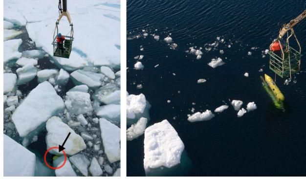
Figure 3: The size of open leads and density of the ice during AUV recovery varied greatly from dive to dive. Opening a pond sometimes also required moving the ship, temporarily precluding AUV communications. The AUV is barely visible in the left image.
