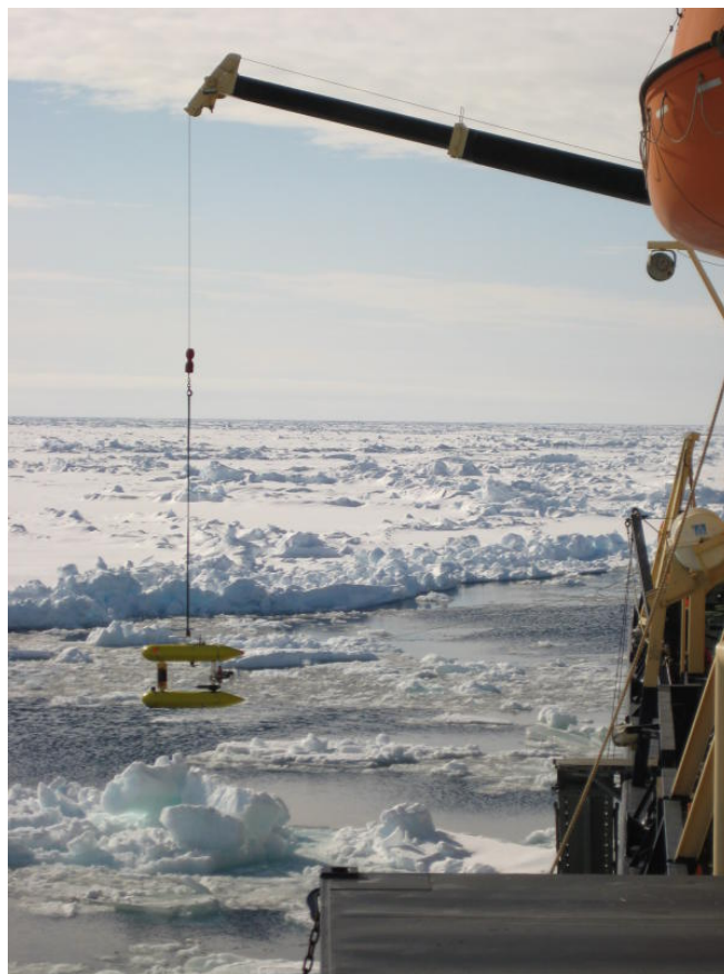
Fig. 1. A typical deployment scenario for the AUV consisted of an open lead or pond into which the vehicle was released. The leads often contained large broken pieces of ice.
