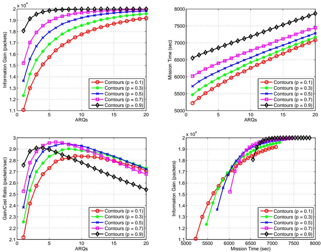
Fig. 3. Simulations of an AUV collecting data from an underwater sensor network. Averages are over 100 random deployments in a  $1 \text{ km} \times 1 \text{ km}$  area with 100 nodes. The AUV executes a data collection tour found using a TSP with neighborhoods. The simulations are performed with varying neighborhood size and number of ARQs.
