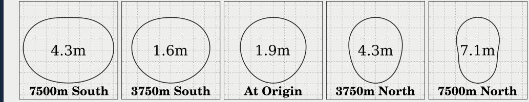
Region adial error in range circles can lead to significant error in computed vehicle locations using LBL. As shown below, this error is magnified near the baseline between two ranging beacons. The rest of the figures on this page show specific calculated range and location errors for an AUV expedition at 85°N latitude.
